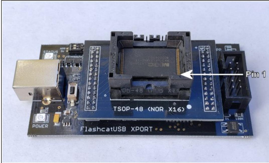
**XPORT PCB 2.0 with the TSOP-48 NOR Socket**
