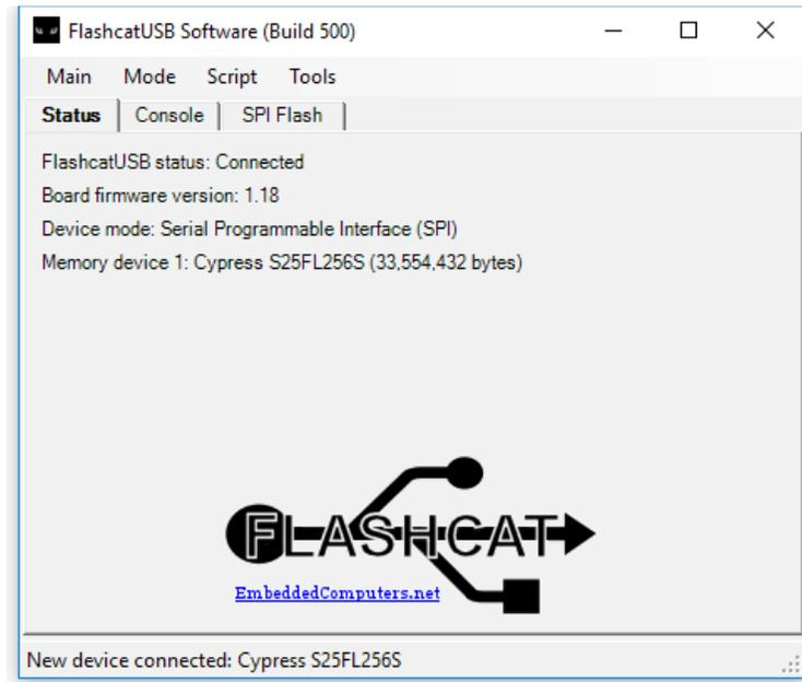
The open-source software will run on Microsoft Windows operating system from Windows XP to newer. If you already connect FlashcatUSB to your PC, when you run the software it will automatically attempt to connect to any attached Flash memory (using the operation mode last used). Otherwise, connect your device, set the operation mode and then click the Detect Device menu option.
