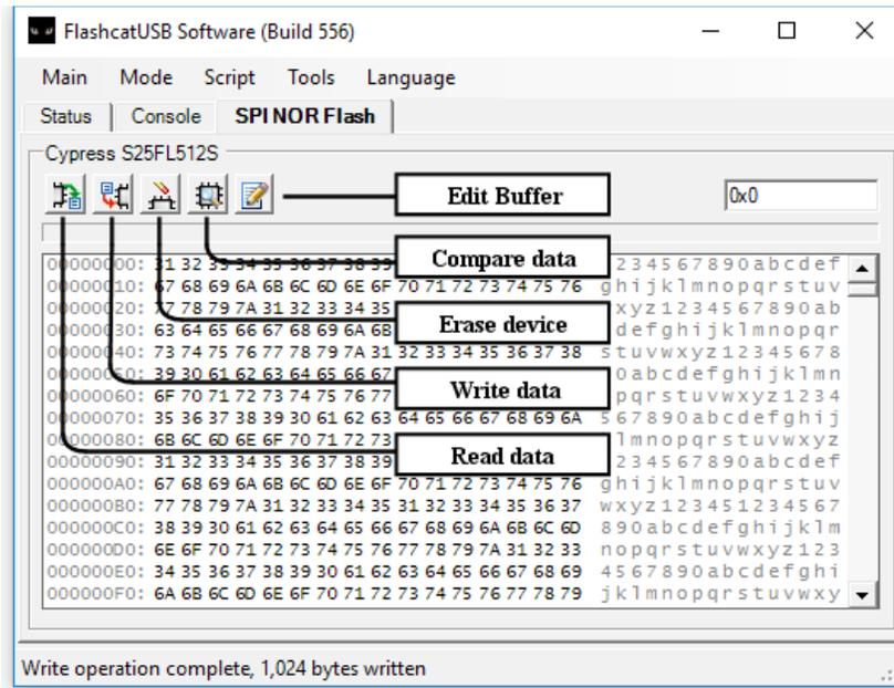
With a Flash device successfully detected, the software will create a Flash tab. This is the primary tool you will use to interact with a Flash device. This window will show you the name of the Flash device, as well as a hex data grid (and ASCII window) representation of the current data on the device. You can scroll down to see the data update in real-time. (Tip: pressing F5 will refresh the screen)
