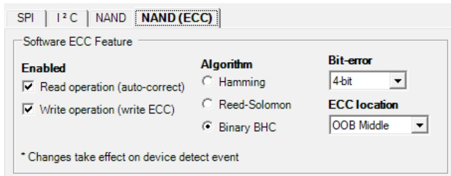
To enable this feature, open up the Settings tab (Mode-->Protocol Settings) and go to the NAND (ECC) tab. Here you can select to use the feature on Read operations and/or Write operations.
