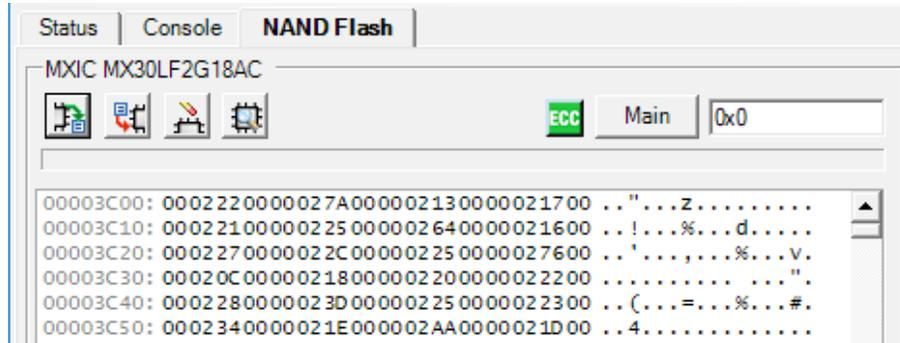
When this feature is enabled for Read operation, the NAND Flash tab can be used to see this feature in action. The icon next to the area selector button will appear. When this icon is GREEN, it means that the software is able to correctly load the ECC data from the Spare area and that the data being show has been corrected (if needed). If this icon is BLUE, it means ECC data was not found and therefore is unable to auto-correct the read operation.
