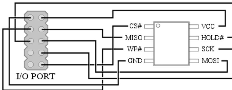
The above diagram is how you should connect the 10-pin port to a typical SOIC-8 and DIP-8 package of a SPI compatible Flash device.
