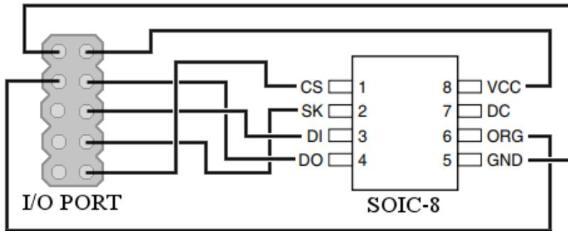
After connecting the device as shown above, open the software and goto the Mode-->Protocol Settings. Then select the MISC tab.
