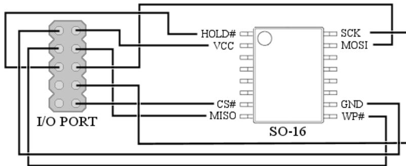
The above diagram is how you should connect the 10-pin port to a typical SOIC-16 package of a SPI compatible Flash device.
