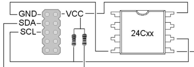
The wiring connection only uses 4 pins from the FlashcatUSB I/O port. When connecting to an EEPROM device, the SDA and SCL lines must also have a resistor that connects to VCC. We recommend using 4.7K values, although any resistor from 4K to 10K should be suitable. If you are using the SPI DIP (revision 2) adapter, you do not need any resistors, as the adapter already contains them.
