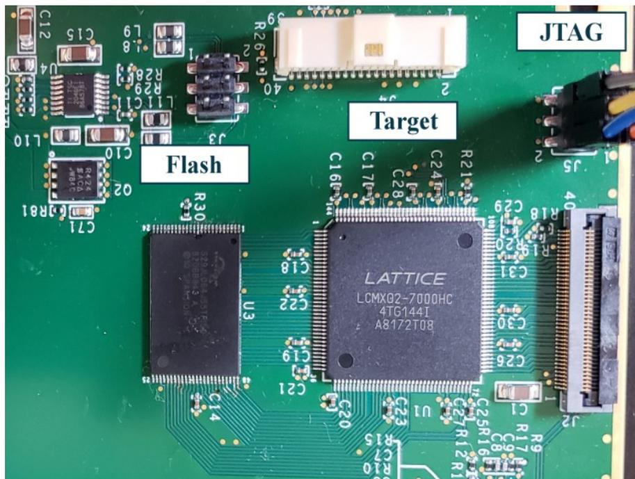
The benefits of using this feature is that the external hardware does not need any special configuration or specific JTAG registers in order to program the memory and is considered the most versatile and universal method. However there are drawbacks. First, data transfer speeds are going to be slow. For example, with the JTAG clock set to 20MHz you should expect a read speed of 5KB/s and a write speed of 2.5KB/s.
