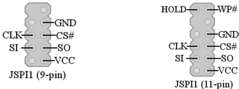
MSI motherboards have a 2mm header labeled "JSPI1". Even though this port is often omitted from the manual, you can connect FlashcatUSB to this header to program the memory. Remember to connect the SO pin from FlashcatUSB to the JSPI1 SI pin, and the SI pin from FlashcatUSB to the JSPI1 SO pin. There are two variants of this header, a 9-pin and a 11-pin. The only difference is with the 11-pin version you will need to connect an additional VCC connection to the WP# pin.
