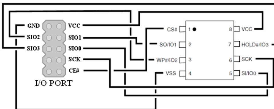
This diagram shows how to connect FlashcatUSB to a Quad I/O (SQI) capable Flash device (SO8 package).
