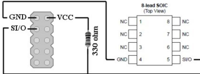
You will need to connect a 330 ohm resistor to the SI/O line and the VCC. For VCC make sure the 3.3V switch is set.
