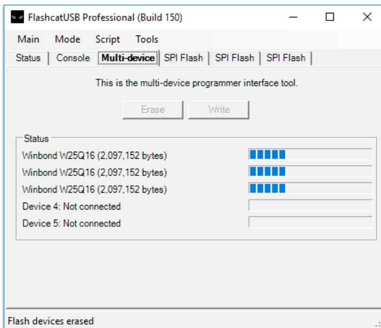
When two or more FlashcatUSB are connected, the software will display the “Multi-device” tab as shown above. From this tab, you can erase or write to all detected memory devices at once. This is ideal for production environments that need to program hundreds, or even thousands of memory devices daily.
